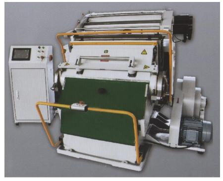
Yawa 720mm x 1040mm Auto / Hand Platen Press Foil blocking + Embossing + Cutting & Creasing machine
