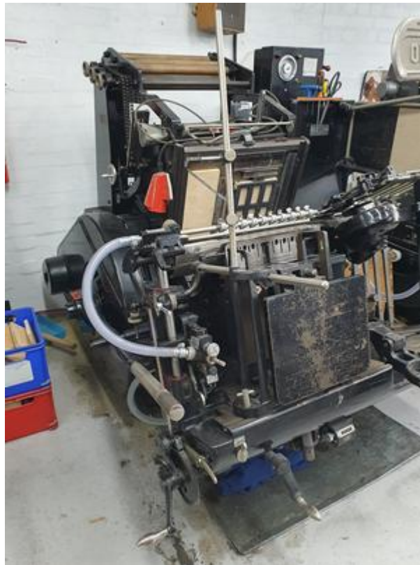
Heidelberg 13 x 18 GTP Platen foil blocking + Embossing + Cutting & Creasing machine
