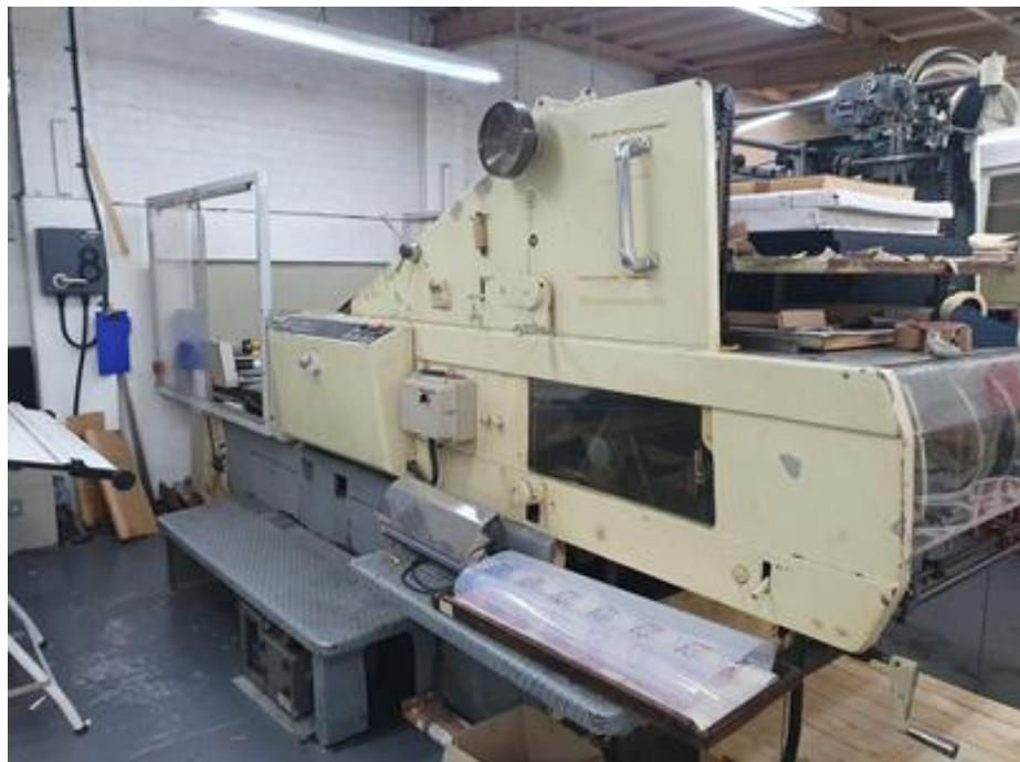
**Miller Johannesburg 104S 720x1040 cylinder foil blocking machine, converted by B&H Machinery.**
