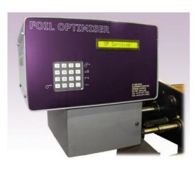
The FOIL OPTIMISER is a replacement for the old original mechanical chain foil pull drive mechanism on a Heidelberg GTP.
