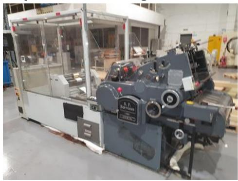
Heidelberg "KSBA" 460mm x 585mm cylinder foil blocking machine that has had the base unit completely refurbished in 2005. New foil pull conversion fitted.
