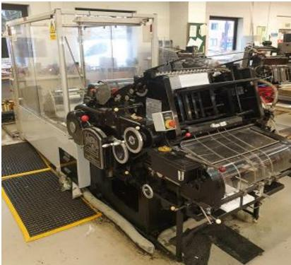
Heidelberg "KSBA" 460mm x 585mm cylinder foil blocking machine that has had the base unit completely refurbished in 2006. New foil pull conversion fitted.
