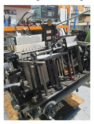
Heidelberg "T" 10"x15" (26cmx38cm) Platen foil blocking machine that has had the base unit partially refurbished. New foil pull conversion fitted
