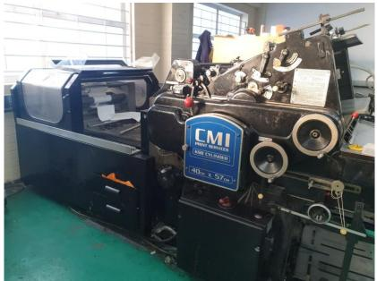
Heidelberg "KSB" 400mm x 570mm cylinder foil blocking machine, refurbished by CMI
