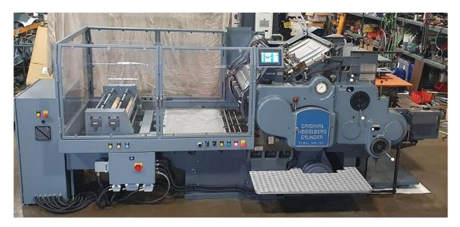
Heidelberg "SBB" 570mmx820mm cylinder foil blocking machine that has had the base unit completely refurbished to a nearly new condition, new foil pull conversion installed.
